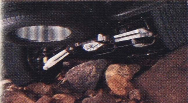
INNOVATION > **02 IRS** > Expedition is the only full-size SUV with a fully Independent Rear Suspension. This new design allows each wheel to respond to the road surface independently for a smooth ride and superb handling.
